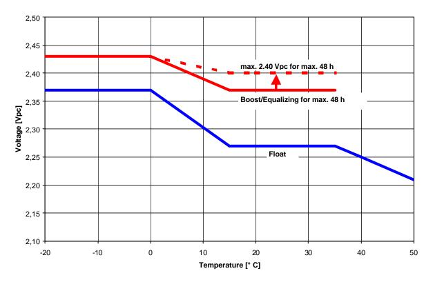
Fig. 3: A 400, Charging Voltage vs. Temperature
