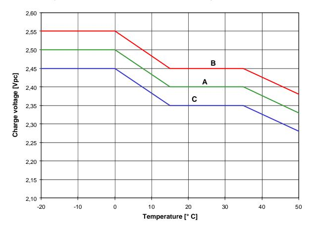
Fig. 17: Charging of Gel-solar batteries depending on charge mode and temperature
