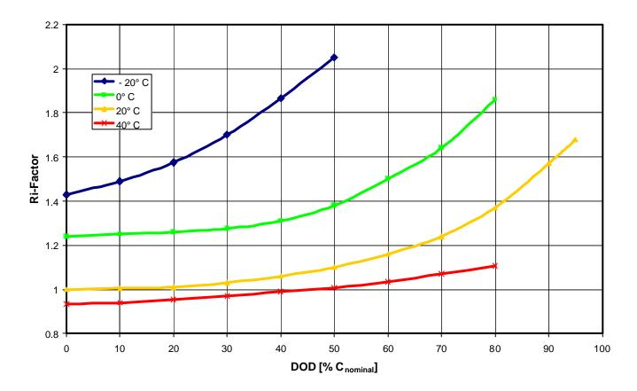
Fig. 18: Internal Resistance R<sub>i</sub> vs. Depth of Discharge (DOD) and Temperature
