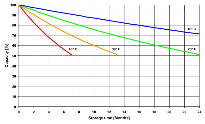
Fig. 1: Self-Discharge vs. Temperature (standard Gel-batteries)
