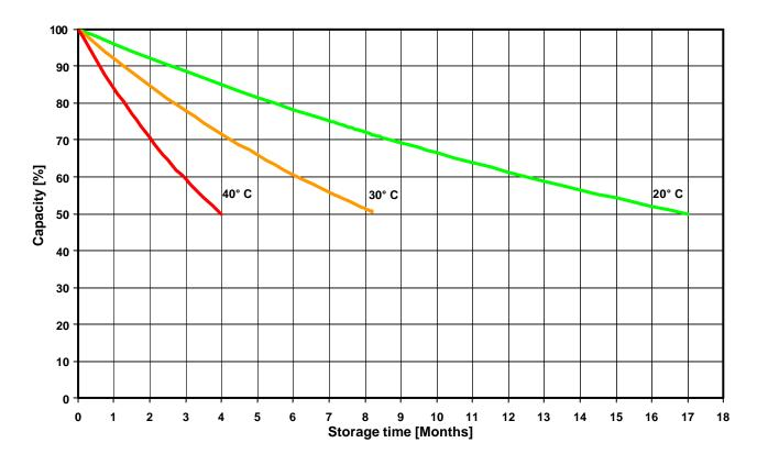
Fig. 2: Self-Discharge vs. Temperature (Gel-solar batteries)
