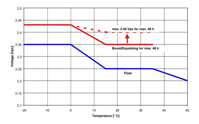
Fig. 5: A 600 and A 700, Charging Voltage vs. Temperature
