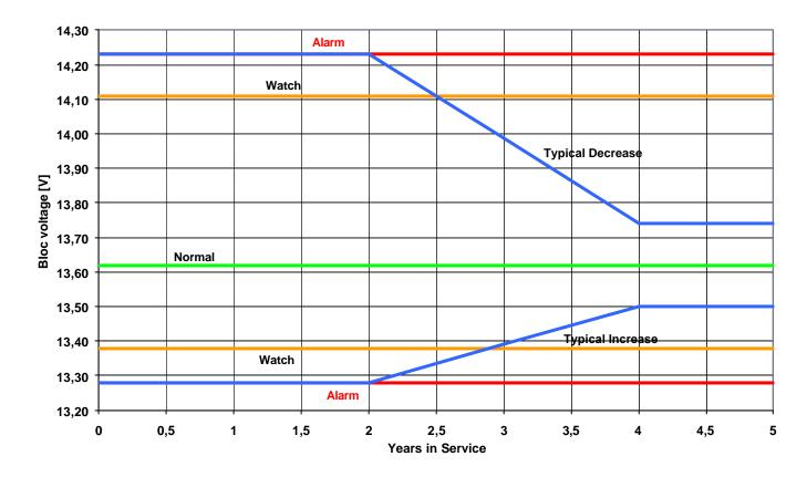
Fig. 8: Float Voltage Deviation in A 400 Batteries (12V-blocs)
