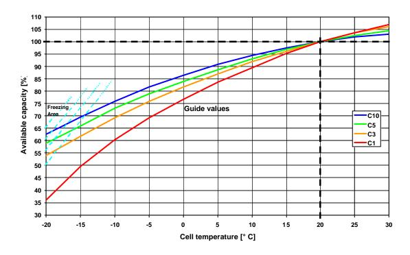
Fig. 20: A 600, A 600 SOLAR, A 700: Capacity (% rated capacity) vs. Temperature
