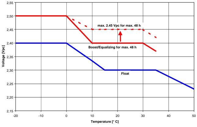
Fig. 4: A 500; Charging Voltage vs. Temperature
